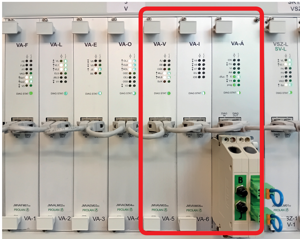
Picture 2: Complete point module (7 cards); in red frame PCBs necessary for reduced point module
